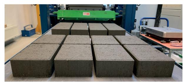
FIGURE 7 - CONCRETE PAVING BLOCKS WITH HALOSEP TREATED FLY ASH
