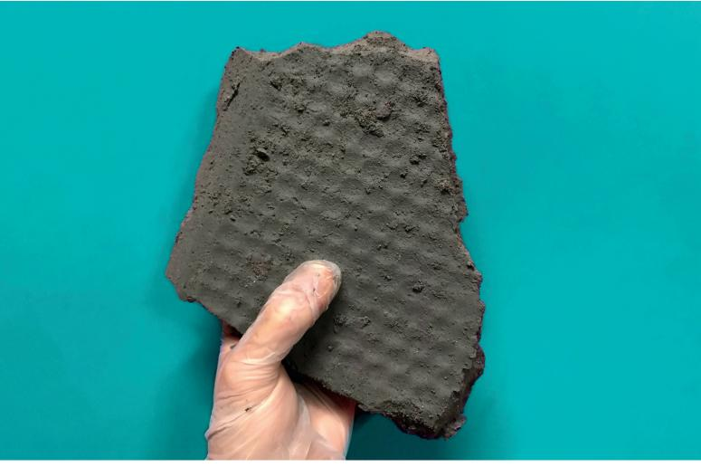
FIGURE 4 - THE TREATED FLY ASH FROM HALOSEP
