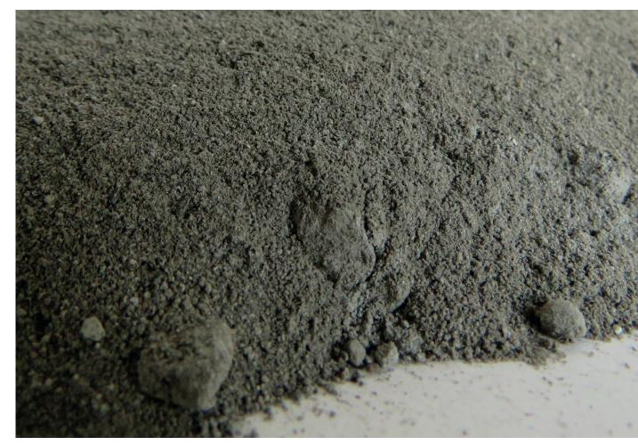
FIGURE 1 - UNTREATED HAZARDOUS FLY ASH
